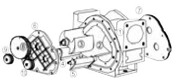
Meter Element Exploded Line Drawing
