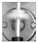
Adjuster drive gear engaged at top
