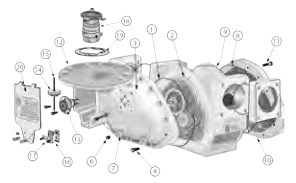
Meter Assembly Exploded View
